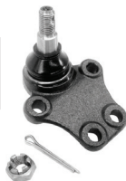
IS1911 Lower Ball Joint (Ø19.6)
