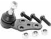
DA1914 Lower Ball Joint (Ø13.3)
