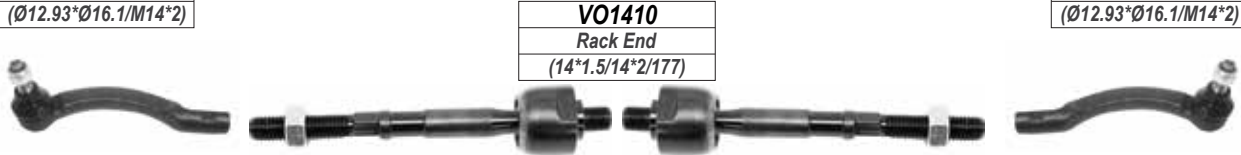
VO1010 Outer Tie Rod End (Ø12.93*Ø16.1/M14*2)
